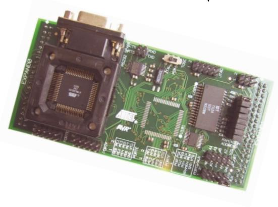
The STK501 board is an expansion module designed to add 64-pin support to the Atmel STK500 Development Board. The STK500 and STK501 expansion module extends support to all current AVR devices.
